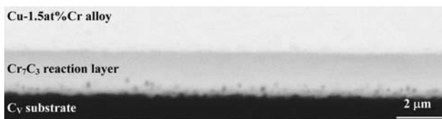
Fig. 4 Scanning electron micrograph of a cross-section through a drop of Cu–1.50 at.% Cr/C v interface at the center of the drop after spreading at 1,150 °C on vitreous carbon followed by rapid cooling (about 3 K/s)
